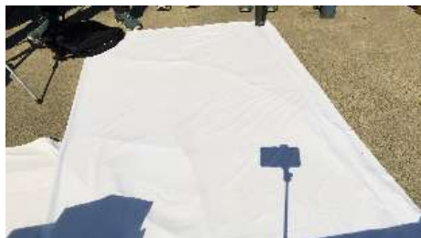
Figure 1: Eclipse shadow band experimental setup at the 2024 Eclipse 2 . This image contains shadow bands that, while difficult to see in the image, are detectable by the human eye during an eclipse and become clear after image processing.
