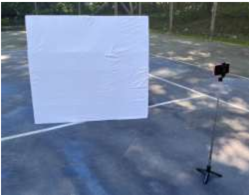
Figure 3: Experimental setup for the August 12, 2026, eclipse. Four cardboard boxes are taped together to form a large observation board covered with a white bed sheet or white poster boards. The board is held in place by a fifth cardboard box. The board is positioned near perpendicular to the Sun, which will be low on the horizon near sunset.
